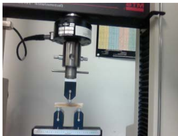
Figure 3. Instron Universal Test Machine set up for flexural testing
