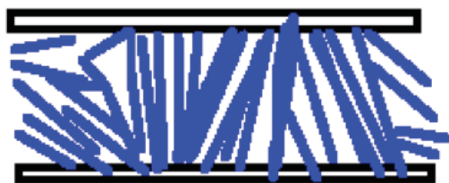
Figure 5: The actual freezing direction of the 1-0-1 horizontally frozen samples.
